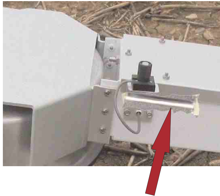
The IRGA measuring chamber is located next to the soil sample chamber
