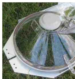
Transparent Open System with pressure equalization valve
