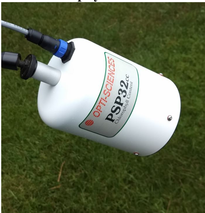
Automated daylight dark adaption for chlorophyll fluorescence
