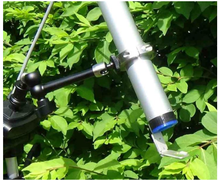
Standard chlorophyll fluorescence probe
