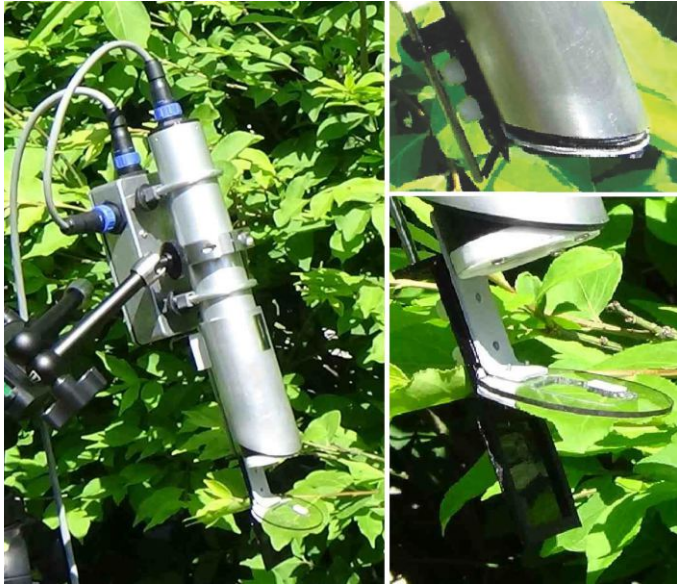
Automated daylight dark adaption for chlorophyll fluorescence
