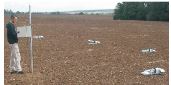
The ACE Multiplexed System Stations may be 200m apart.
