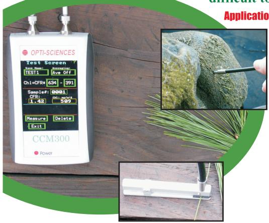
The CCM 300 Uses a proven fluorescence ratio technique for chlorophyll content measurement.
